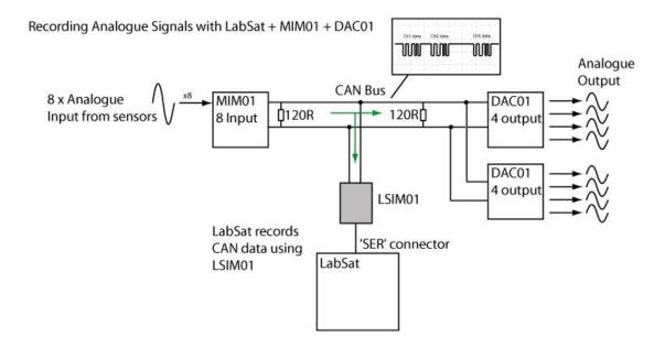
"To accurately replay the analogue data simultaneously with the GPS RF data, the CAN Interface Module converts the digital information back into CAN data, which is replayed synchronised with the GPS RF data. The CAN data is converted back to analogue data using a Racelogic Analogue Output Module."
