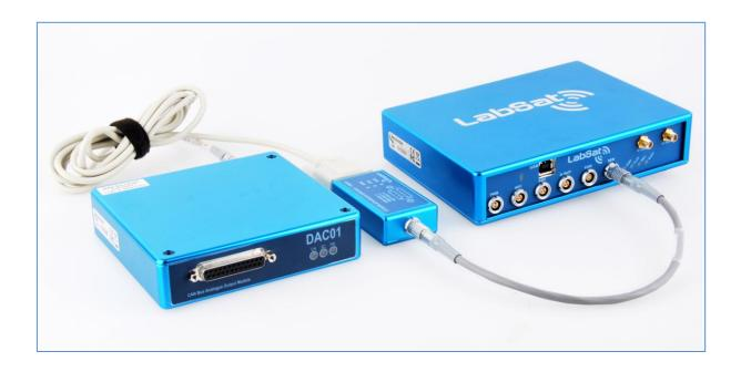
Racelogic have announced that their LabSat GPS simulator now has the ability to record and replay analogue signals too. This is good news for navigation system and inertial integration developers, as it's now possible to test synchronised data from external sources alongside GPS.
