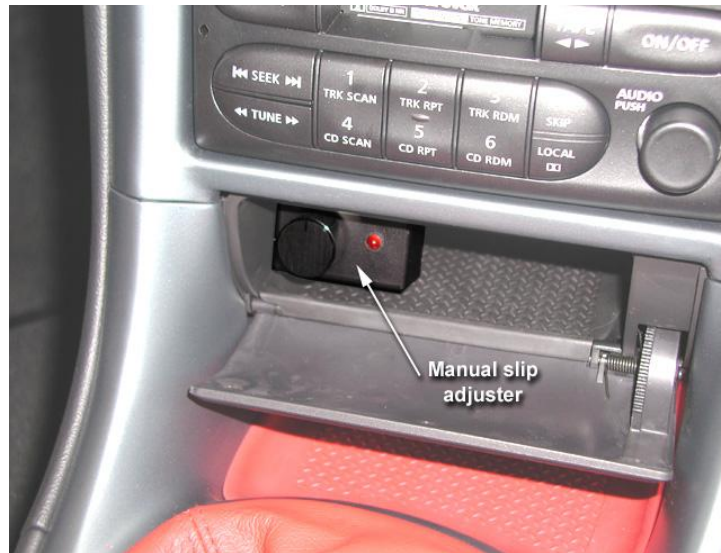
Manual Slip Adjuster installed in a Holden HSV
