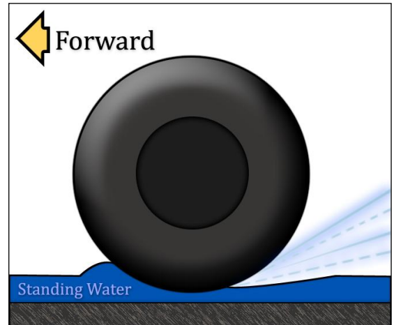
Water on the road which cannot be displaced causes aquaplaning
