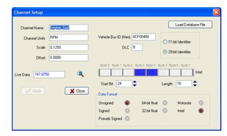
The byte position display corresponds to the 8 bytes in a CAN message. As the start bit and length are changed, this display will update to give a visual confirmation of the data source.
