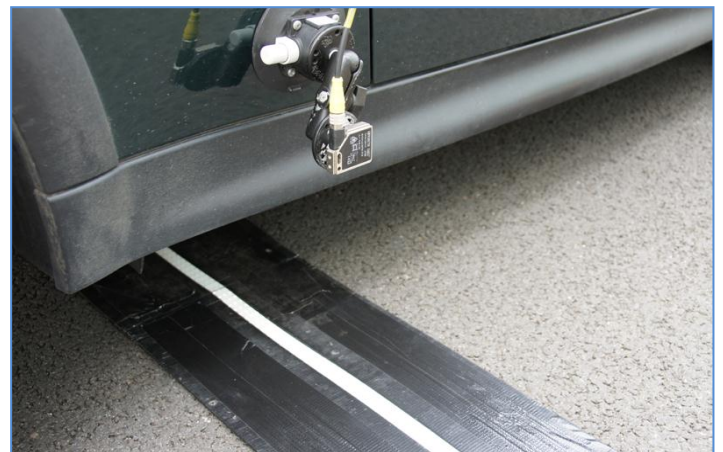
Fixed starter point with laser range finder
