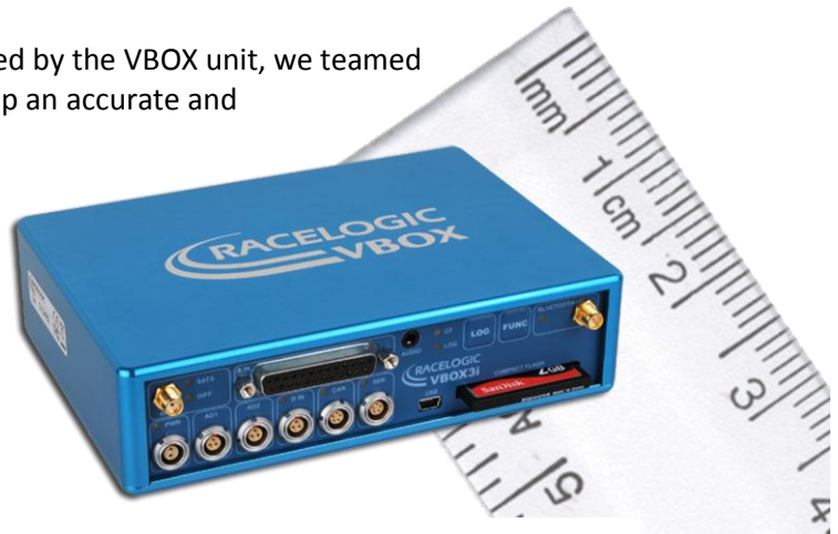
VBOX 3i accurate to within \pm 2\text{cm}
