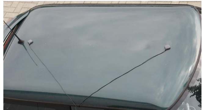
Two antennas fixed to the front and rear of the vehicle with two VBOX 3i devices
