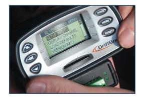
**7.** The values on the screen are probably different to the actual speed at which the engine is running, and will need to be scaled to display the correct RPM value. To do this, press the **MENU** button.
