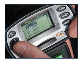
**8.** Select the channel that you wish to edit – in this case, the RPM channel.
