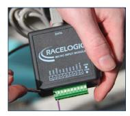
**4.** Connect the **MICRO INPUT MODULE** to your data logger (in this case a **DriffBox**), and start the vehicle's engine.
