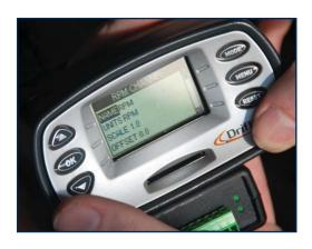
**9.** Using the arrow buttons, scroll down to the Scale option, and press **OK**.
