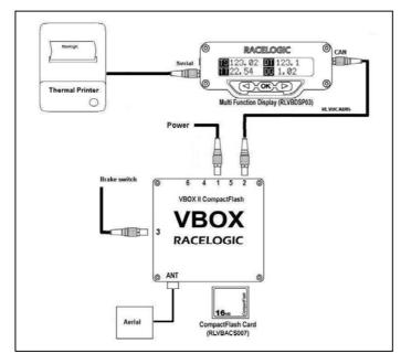
Connect the Multifunction display to socket two of the VBOX using a CAB05 cable and mount the MFD on the windscreen of the vehicle using the suction cup mount. Then connect the Thermal printer to the 'Serial' socket of the MFD. The Brake trigger is plugged into socket 3 of the VBOXII and attached to the brake pedal. Use of the Brake Trigger is only applicable to VBOXII and VBOXIII.
