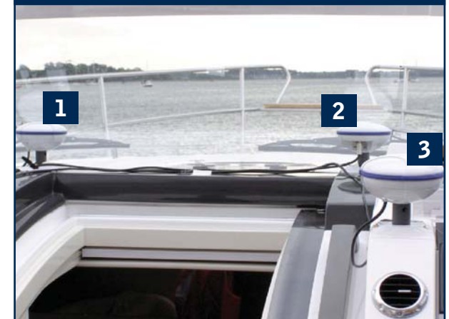
3 x Ground Plane Antennas
