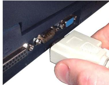
6. Connect other end of USB or serial cable to VBOX
