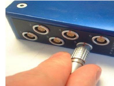
7. Connect the power cable or battery pack to the VBOX
