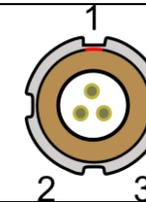
**Connector 5 – CAN (First CAN Bus Connector, Serial Connection to GPS Engine)**
