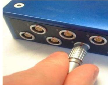
7. Connect the power cable/ battery pack to the VBOX
