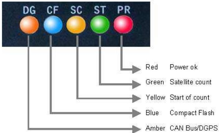
The green LED (**ST**) is used to indicate the number of satellites currently in lock. If the yellow LED (**SC**) is flashing whilst the green (ST) LED is off, then the VBOX has no satellite lock.
