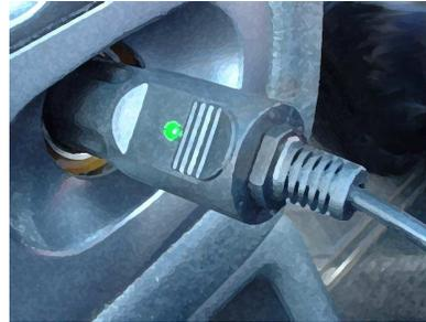
9. With the power applied, the red PWR led should illuminate. The VBOX Pro Lite will start searching for satellites. The Green led will indicate the number of satellites currently in lock. For best results ensure the VBOX has acquired a lock on 5 or more satellites, essential for quality signal reception. When using the VBOX for the first time or when using the VBOX after a long period of time, allow the VBOX to sit for between 5 and 10 minutes to re-collect data needed to track satellites.
