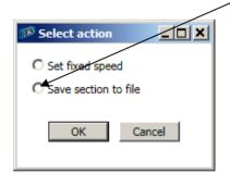
Now do the same thing for section D to A, but this time you can mark the end of the file by doing Shift E. Save this file to say *Section 3.SPD*. Note, Shift E will only mark the end of the file, if the last point has been designated as *Finish* point within point setup.
