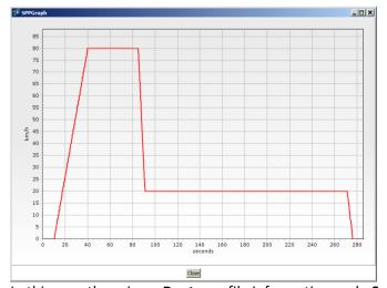
In this case there is no **Route** profile information, only **Speed** profile, so the file is saved as .**SPP** file type. Use **File > Save** to save the file. Once the .**SPP** file has been saved, you are now ready to download the file into the OLED display. See page 22 **COMM Ports**.
