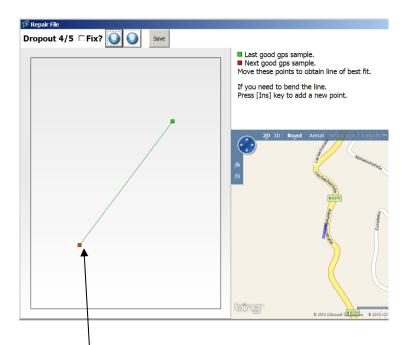
On the left hand side you can see a straight line, indicating the length of the dropout with a green marker showing the **last** good GPS sample, and a red marker showing the **next** good sample. On the right hand side you can see the section of the route where this dropout occurs.
