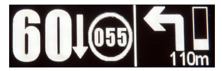
On the left you can see the actual speed of the vehicle with the ideal speed in the circle to the right. There is an arrow indicating slow down or speed up between the two speeds.
