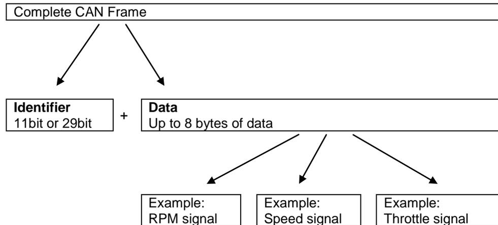
The CAN Display is capable of showing Raw CAN data. Raw CAN data refers to complete CAN frames, showing the identifier and all of the data for each frame in hexadecimal number format.
