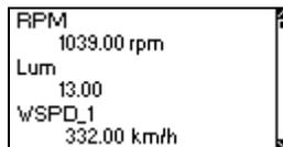
Three signals are displayed at once in a scrollable real-time list.
