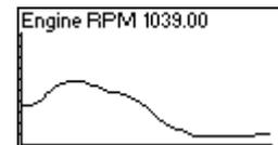
Graph limits are taken from the database. Update rate of the graph is user adjustable in the DBC VIEW menu, accessed by pushing the button. Rotating the adjuster will switch between each DBC signal in the current database.
