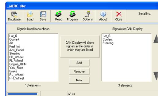
By double-clicking on a signal in the right-hand list, it is possible to display and make changes to the signal settings. This can be useful for adjusting the Max and Min Values for the signal, which are used as the graph limits when the CAN Display is in graphical mode. Click “Apply” to record any changes that are made then close the Signal Details window.
