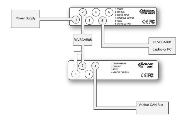
Using the 5 way LEMO to 5 way LEMO cable (RLVBCAB05) connect socket 2 (CAN BUS) of the VBOX to socket 1 (CAN/POWER IN) or socket 2 on the CAN02 module. Power the VBOX using either the mains adapter or a fully charged battery pack. Connect socket 5 (RS232) of the VBOX to COM2 or COM2 on a PC
