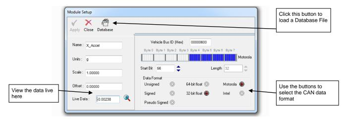
It is also possible to import industry standard CAN database files with the ".DBC" file extension or to purchase encoded data set files from Racelogic with the .REF extension. These files contain CAN data signals that have been recorded by Racelogic to provide basic functions for most makes of vehicle. Most of the data sets will contain at least the following signal parameters:-
