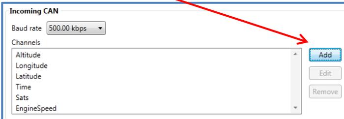
The CAN database can now be expanded to reveal all of the CAN channels available.
