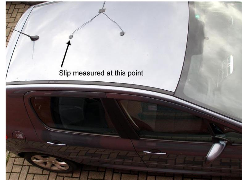
**Antenna A** is the *primary antenna*, from which all calculations are based. If overall slip is to be measured (at the centre of the vehicle), the primary antenna should be placed rearward of the secondary. Alignment of the antennas is not completely essential as the Slip Angle Sensor has the ability to calculate any offset. See the Slip Angle Offset Section.
