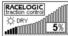
Turning the selector will move the settings 1% at a time and the unit will default to the last setting on power up. The slip level range is from 0% - 25%. In order to turn Traction Control off the selector needs to be turned to 25% when after two seconds the following screen will appear:
