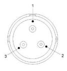
3 PIN LEMO PLUG VIEW FACING PINS LEMO PART NO. FGG.0B.303 CLAD52Z
