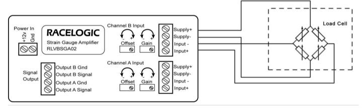
The Strain Gauge Amplifier can also be used in half-bridge and quarter-bridge applications. Please refer to the user manual for more information.
