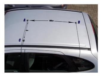
Based on the successful twin antenna VBOX IISX (RLVB20SL) design, the triple antenna VBOXII SX (RLVB20SL3) incorporates a third GPS channel to allow users to measure simultaneous angle measurements along 3 axes. As a small sized unit with simple installation procedures and a built-in configuration screen, the RLVB20SL3 is ideally suited for use in a range of both land and water vehicles.
