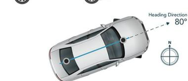
VBOX 3i Dual Antenna is compatible with all existing peripherals, including the Inertial measurement unit which provides a highly accurate speed, distance, heading, and yaw rate measurement for use in ESC testing with a steering robot.
