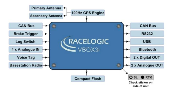
Note: On a VBOX 3i RTK the 'SL' and the 'RTK' features are ticked on the silver serial label. All units with the 'IMU04 ready' sticker can be used for GPS/INS integration using the IMU04.
