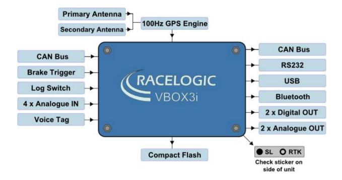
Note: On a VBOX 3i Dual Antenna the 'SL' feature is ticked on the silver serial label. All units with the 'IMU04 ready' sticker can be used for GPS/INS integration using the IMU04.
