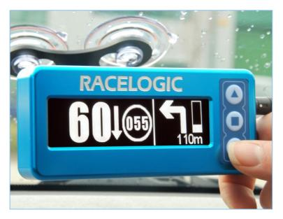
Above: the speed profiler OLED display is showing a speed of 60km/h, and that the driver must slow to 55km/h. The amount of user deviation permitted from the required speed is adjustable. The speed profiler is also stating that the driver must turn left in 110 meters.
