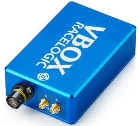
The VBOX 3iS Dual Antenna is RTK (Real-time Kinematic) enabled, offering cm-accuracy when used in conjunction with an RTK base station or other RTCMv3 correction sources such as NTRIP. This enables it to be used as a moving target, as part of a VBOX ADAS setup, or with a steering robot, to which it can connect via Ethernet.
